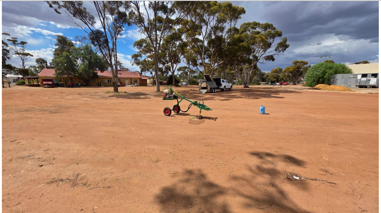
Photo 03: Subsurface probing by hand auger at Borehole BH2 location
