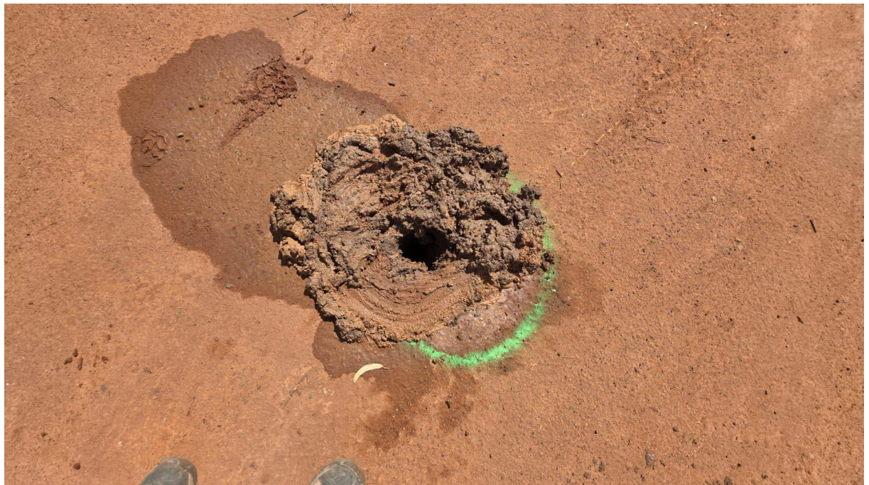
Photo 03: Subsurface probing by hand auger at Borehole BH2 location
