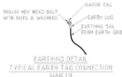
EARTHING DETAIL TYPICAL EARTH TAG CONNECTION SCALE 1:10
