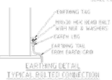
EARTHING DETAIL TYPICAL BOLTED CONNECTION SCALE 1:10
