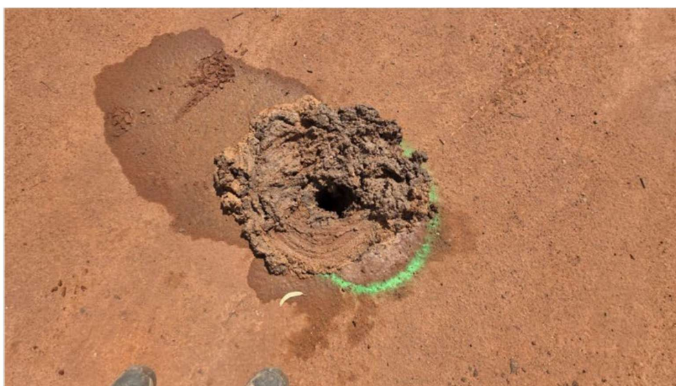
Photo 03: Subsurface probing by hand auger at Borehole BH2 location
